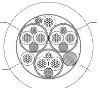
Overall screen comprising polyester/aluminium laminate tape, tinned copper drain wire
