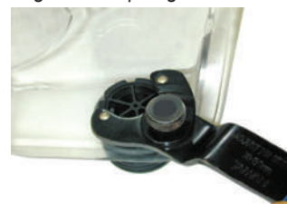
Figure 7. Seat Valve removal
