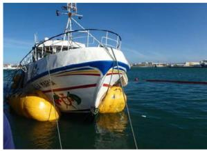
For shallow water and surface floatation, draft reduction and towing, Totally Enclosed Cylindrical bags are ideal for general lifting and buoyancy provision. Remote inflation and deflation increases safety and provides lifting options for a wide range of applications.
