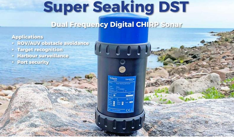
The V7 Super SeaKing DST mechanical scanning sonar now offers enhanced performance and the option of Ethernet communication for high speed scanning over short ranges. Retaining dual frequency capability, the Super SeaKing DST can achieve 300 m range at 325 kHz, with increased image intensity and with improved mid-water target discrimination capability at 650 kHz.
