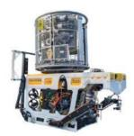
Top Hat style Tether Management System with a 400 m winch module for a 20 mm tether fitted with latch status and line out sensors. Options include lights and cameras.
